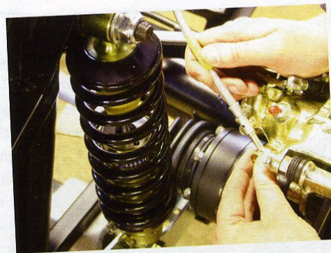
Rear flexi pipe being fitted.
