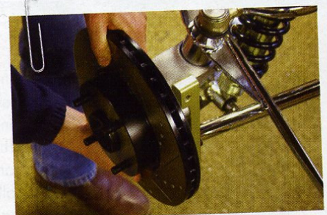
step 2: sliding the ventilated disc over the studs.
