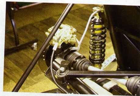
Handbrake cable in place. Note how neatly it is attached to the De Dion beam.
