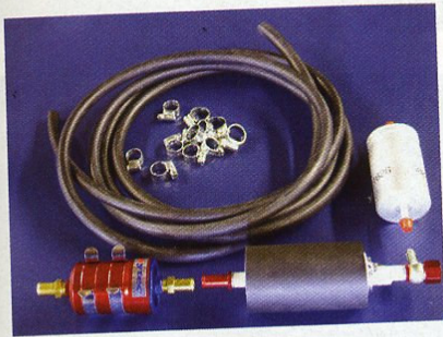
Fuel pump, filters and pipe.
