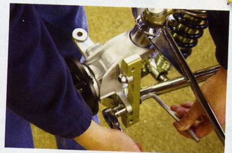
step 1: fitment of the billet alloy mounting bracket.
