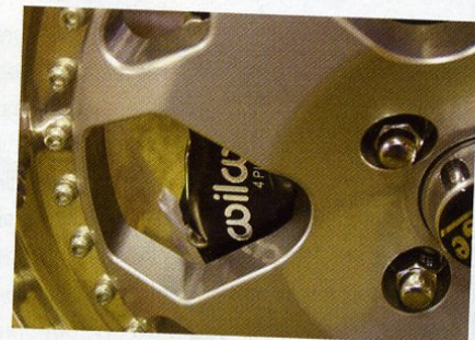
Note the minimal clearance to the Wilwood racing callipers.
