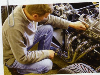
Exhaust system bolted to Merlin heads. Nigel, seriously relieved they missed the chassis members.
