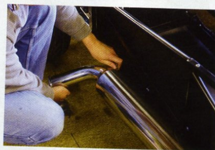
Tailpipes attached to chassis using rubber mounts.
