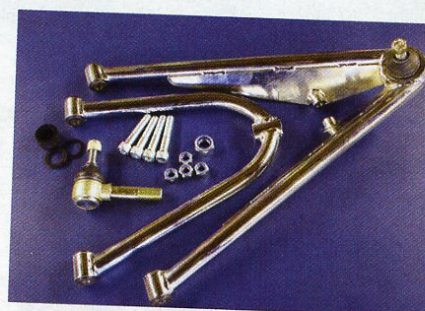
Front suspension components for passenger side. Note chromium-plated wishbones, a typical DAX upgrade.
