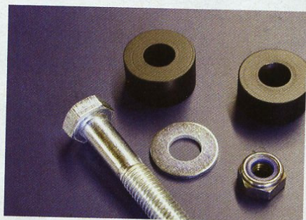
Spacers turned up on Nigel's father's lathe to accommodate differential in chassis.
