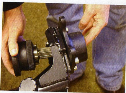
De Dion tube in place. Here you can see the splined stub axle being passed through the bearing carrier.
