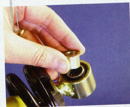
Top hat reducers allow M12 suspension bolts to fix shocks securely.
