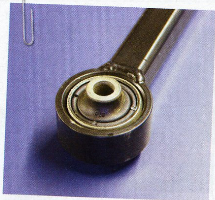
Large rubber bush pressed into one end of the De Dion 'A'
