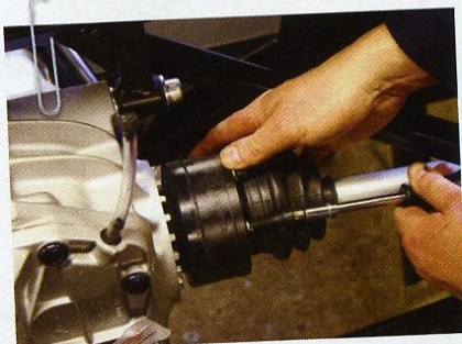
Lobro joint being fitted to the differential using brand new Torx bolts.
