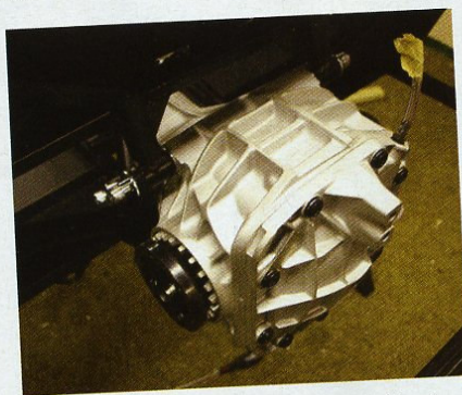
Rare fully reconditioned 3.36 ratio differential in situ.
