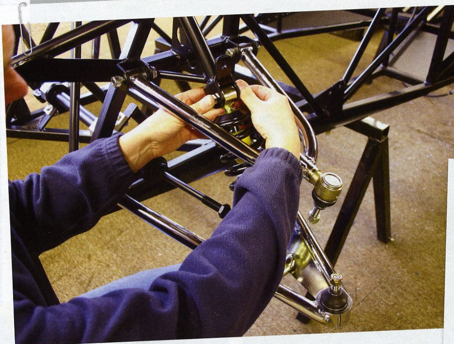
Top wishbone in place, next the shock absorber and spring.
