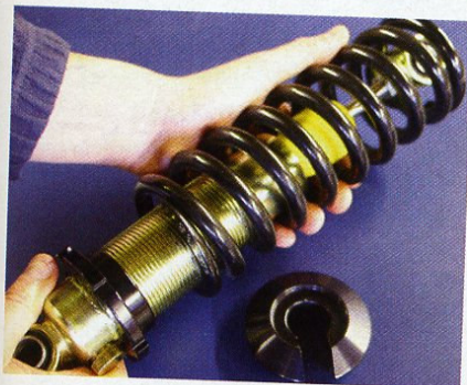
Springs being passed over GAZ shocks.
