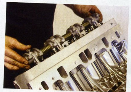
Rocker shaft assembly being bolted to the merlin head.
