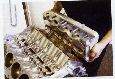
On go the Merlin F85 heads, one of the secrets to the Raptor's astonishing capabilities.
