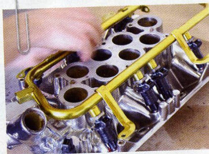
Injection inlet manifold being assembled. This is actually a dummy run as the inlet ports still need to be opened out to maximise gas flow.
