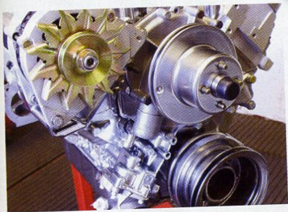
Pulley set-up in place. Will the alternator fit in the Rush chassis?
