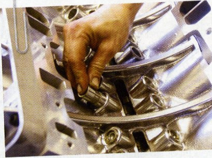
Hydraulic followers being inserted into the V8's valley.
