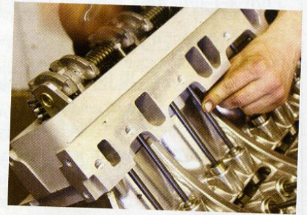
Adjustable push rods being inserted prior to adjustment.
