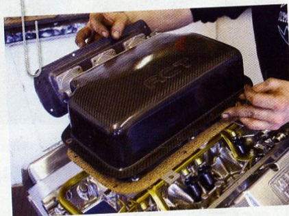
On goes the ACT carbon fibre triple throttle body plenum. Absolutely exquisite.
