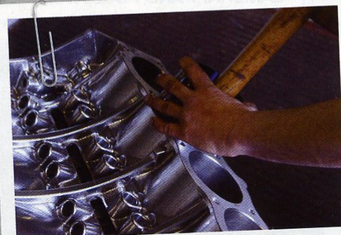
Using a ring compressor to insert all eight pistons into the COSCAST block.
