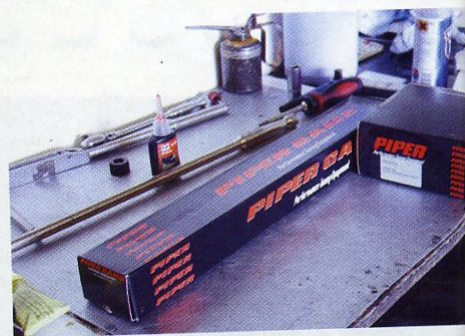
Piper 285 camshaft and hydraulic followers.
