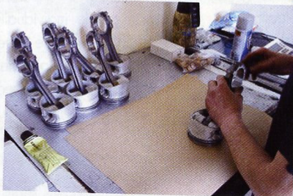
Pistons and end caps being prepared for insertion.
