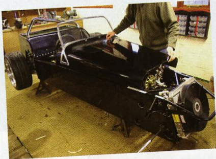
Trial fit of bonnet ... whoops! Even with the plenum removed it will not sit home.
