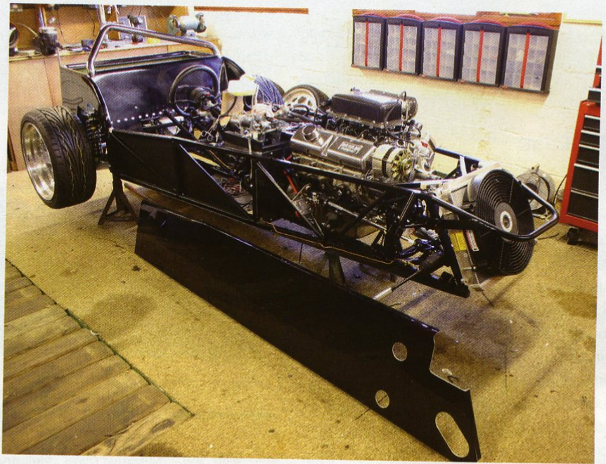
Driver's side panel awaiting initial fit.
