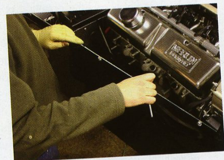
Accurate fitment of side panel to top chassis rail.
