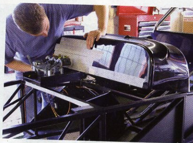
Marking scuttle to allow for pedal box.
