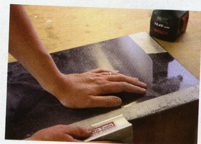
Filing block removes any carbon fibre shards remaining after cutting.
