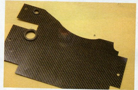
Driver's tunnel end in carbon fibre. This complex shape took a good few hours to create.
