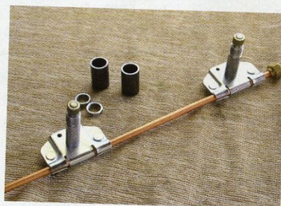
Wheel boxes prior to insertion in scuttle.
