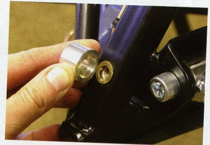
Machined spacers to ensure radiator is firmly positioned away from chassis rails.
