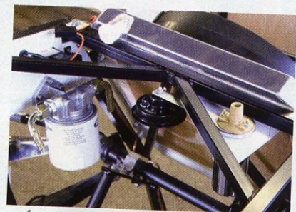
Fan controller and coil brackets bolted to chassis.
