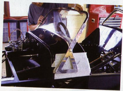
Nigel lining up windscreen prior to drilling fixing holes.
