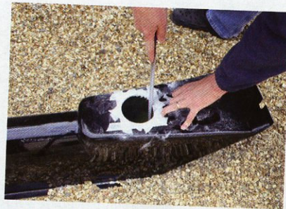
Creating hole in centre console for Tremec gearstick.
