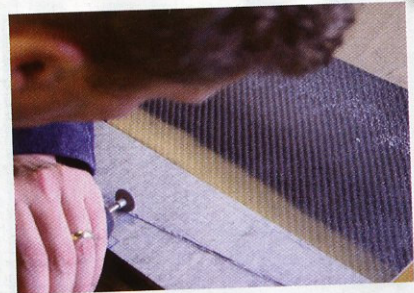
Cutting carbon fibre sheet with a Dremel and special Perma-Grit disc.
