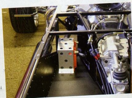
Battery positioned at end of passenger tunnel. This will be panelled in due course.
