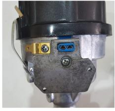
Next connect the blue and red wires that come from the grey shielded cable on the distributor side of the RPi A&R Amplifier as follows.
