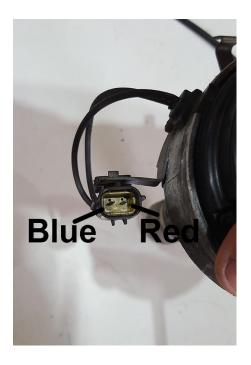
Those amongst you that are paying attention will notice that this means our amplifier connections on this distributor plug are the other way round to the blue and red wires on the plug that you removed. Don't panic, there is no need to call us, this is correct.
