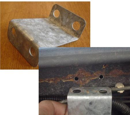
At this point I also bent the bracket ready for the Power boost valve to be fixed to it. As seen above.
