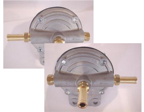
The input pipe is the one coming from the side of the Power boost valve and is going to be connected to the adaptor plate. As you can see I have had to change my one for this Range Rover from one side to the other.
