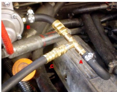
As seen above. Point A was connected to the power boost valve but is now joined to the pressure gauge T-piece. Point B is now connected to the power boost valve so that the fuel is still flowing on its original path. Point C is going off to the Gauge.
