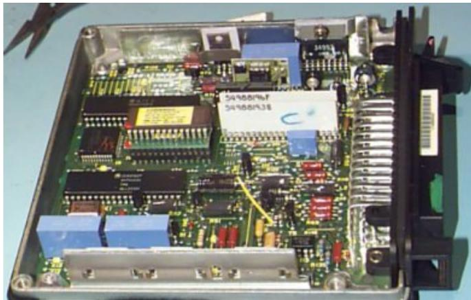
Ensure that the correct Tune Resistor is fitted to the vehicle. This will be marked on the ECU and EPROM chip labels, and varies according to application.
