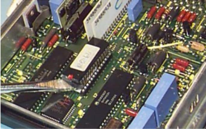
Now the EPROM itself may be removed as follows, again as shown in the picture on the left. Gently lever it out by placing a thin screwdriver blade between the chip and socket, and rotate the tip to prise it out.
