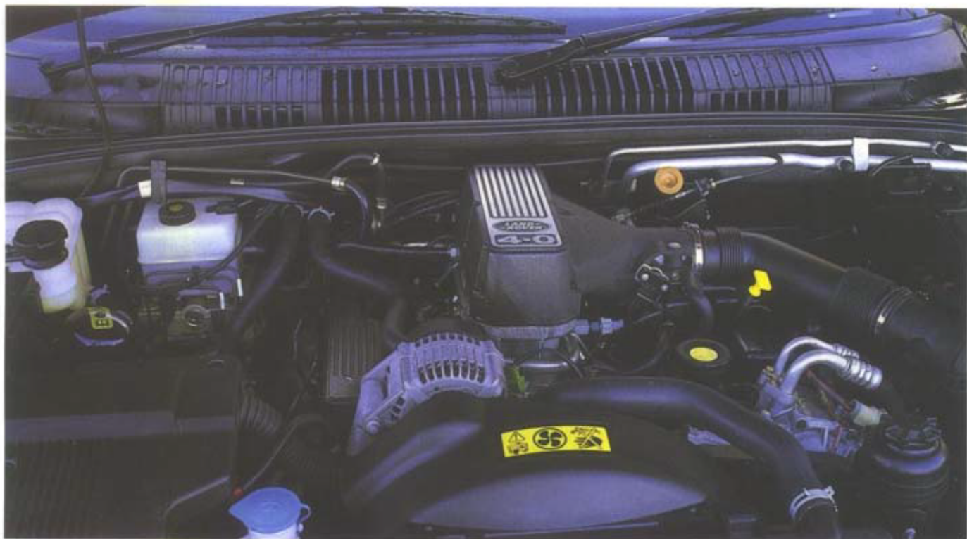
Out of all the later long-stroke V8 motors, the 4.0-litre unit (above) appears less prone to cracking than the higher-torque 4.6-litre engine
