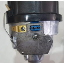
Next connect the blue and red wires that come from the grey shielded cable on the distributor side of the RPi A&R Amplifier as follows.
