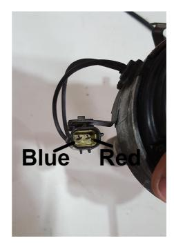
Those amongst you that are paying attention will notice that this means our amplifier connections on this distributor plug are the other way round to the blue and red wires on the plug that you removed. Don't panic, there is no need to call us, this is correct. **Metalic amplifier box mounted near to the coil and purple and orange wires from the dizzy** These are not so common however we do still see some out there (although by now the mechanical advance curve could probably be questioned)
